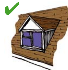
Gable-Ended Dormer Roof
