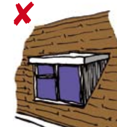
Flat Dormer Roof
