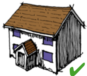
Gable-Ended Pitched Roof
