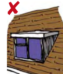
Flat Dormer Roof
