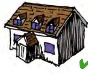
One and a half Storey with Pitched Roof Dormers to enhance Appearance
