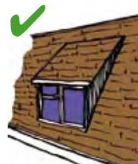
Cat-Slide Dormer Roof
