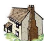
Typical Lean To Porch and Chimney
